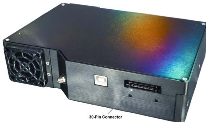
Location of QE65000 30-Pin Accessory Connector
